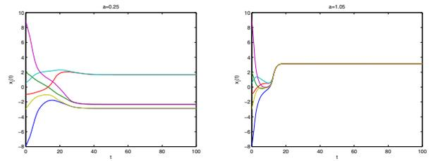
Fig. 2. Simulation of the first scenario. For weak coupling and initial data that converge to different equilibria, there is not convergence to a common value. Here  $a = 0.25$  does not satisfy the condition of Theorem 4.2. Stronger coupling  $a = 1.05$  does satisfy the condition of Theorem 4.2 and it leads to consensus.
