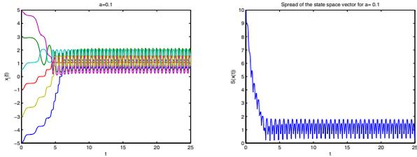
Fig. 4. Simulation of the third scenario. There is no chance for complete synchronization. The stronger the coupling is, the smaller the  $S(\mathbf{x}(t))$  becomes, as  $t \rightarrow \infty$ . Here  $S(\mathbf{x}(t)) < 2$  as  $t \gg t_0$ .
