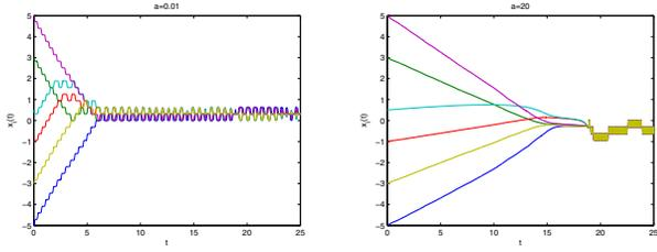
Fig. 3. Simulation of the second scenario. For weak coupling and initial data that converge to different equilibria, there is not convergence to a common value. The situation changes for strong coupling. Due to the non-autonomous nature of the dynamics, the agents converge to a non-constant synchronized solution.
