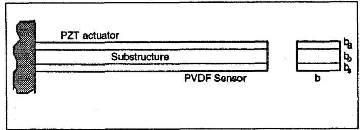
Figure 1: The composite beam
