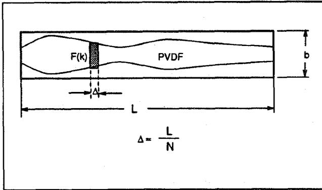
Figure 3: Discretizing the sensor and actuator layout
