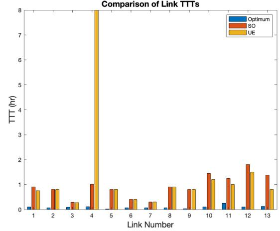
Fig. 2. Comparison of the optimum and calculated TTTs via SO and UE
