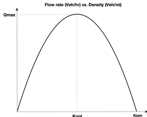
Fig. 1. Concave Estimate of Fundamental Diagram
