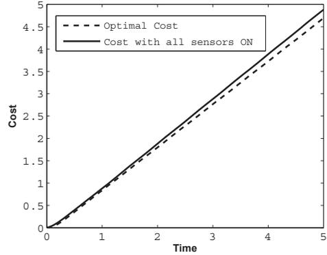
Fig. 2. Optimal cost versus cost of operating three sensors simultaneously.
