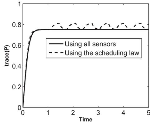
Fig. 3.  $tr(P)$  for optimal scheduling and for the case when all sensors are active.
