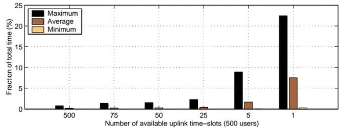
Fig. 9. Percentage of total time BER target is not met by a user as a function of number of available uplink time-slots (500 users)
