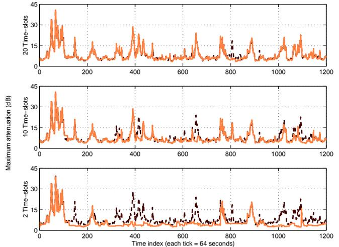
Fig. 4. Time-series plot of actual channel attenuation level (dashed-line) versus the level calculated at the NOC (solid-line) for a set of 200 users
