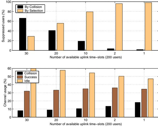
Fig. 5. (a) Fraction of the users suppressed by the FIS algorithm as a function of the number of available uplink time-slots (200 users). (b) Channel usage profile as a function of the number of available uplink time-slots (200 users).
