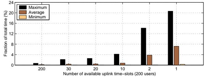
Fig. 8. Percentage of total time BER target is not met by a user as a function of number of available uplink time-slots (200 users)
