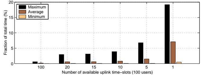
Fig. 7. Percentage of total time BER target is not met by a user as a function of number of available uplink time-slots (100 users)
