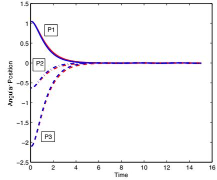
Fig. 2. The red curves show the behavior under continuous feedback and the blue ones for event based feedback. P1, P2 and P3 correspond to pendulum 1, pendulum 2 and pendulum 3 respectively.
