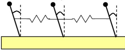
Fig. 1. Three pendulums interconnected by springs. The angular positions are measured anticlockwise from the vertical axes. [12]
