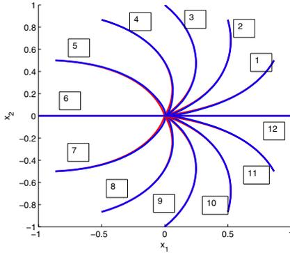
Fig. 4. The red curves are for the continuous feedback system and the blue curves are for the event based system. All the trajectories converge to the equilibrium point at the origin. There are twelve different initial positions as numbered in the figure.
