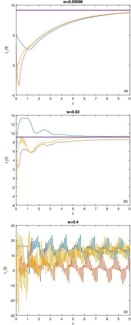
Fig. 3: Simulations run in MATLAB with the `ddesd` routine. The distributed incremental cost solutions  $\lambda_i(t)$  is the consensus variable which appears to converge very fast for small  $w$ . (b) As  $w$  increases beyond  $w^*$  we still see oscillatory and slower convergence. (c) For  $w$  large the algorithm does not converge and for even larger values it diverges.
